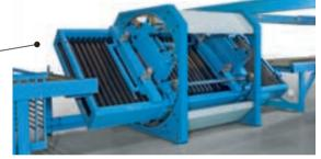
**Turning device TD 6/8** For turning sheared parts upside down for bending etc.
