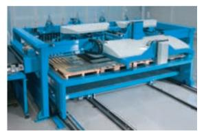
**STS 6/8 stacking system** Automatic sorting and stacking of sheared parts on one or two tables.
